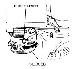
Figure 9. Engine Choke Lever (Closed)
